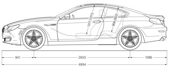
Figures in ( ) apply to the glass vent roof.
